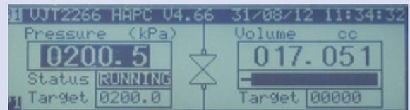
Automatic Hydraulic Pressure controller graphic display. Showing: status, current pressure and volume readings, target values and graphic representation of available volume.
