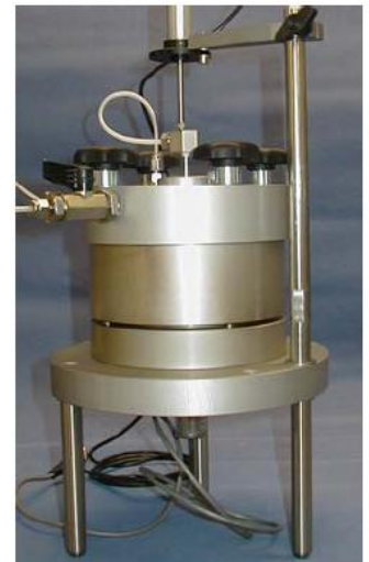
Fig. 4 Cellule de consolidation type Rowe & Barden de GDS.
