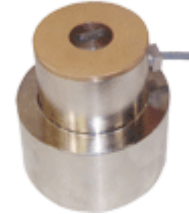
Fig. 2 HAEPD bonded into a bender element triaxial pedestal
