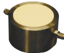
Fig. 1 HAEPD bonded into a standard triaxial pedestal
