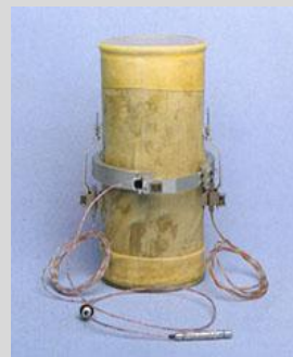
Fig. 12 Hall Effect and LVDT local strain transducers
