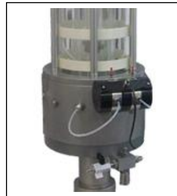
Fig. 8 High accuracy DPT attached to cell
